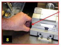
Tighten placement knob to secure aligned position of the blade holder to the CryoAligner tool.
