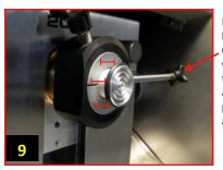
Loosen clamping adjustment knob and remove the CryoAligner tool and replace it with the tissue chuck. Tighten the clamping adjustment knob & the tissue chuck will be in perfect alignment to the base assembly.
