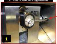
Loosen clamping adjustment knob and remove tissue chuck.
