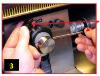
Loosen both the orienting & clamping adjustment knobs to position tool.
