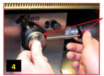
Press the CryoAligner tool flush against back surface and tighten the clamping adjustment knob.
