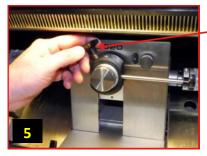
Tighten the orienting adjustment knob to lock in new alignment.
