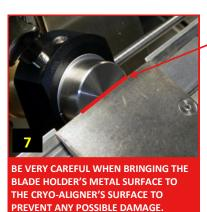
**GENTLY**, bring the blade holder surface against CryoAligner tool's surface so that it is perfectly aligned & flush.
