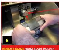
Position blade holder (w/out blade) to start moving towards CryoAligner's front flat surface.
